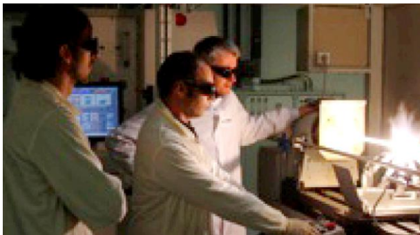
Technicians and Engineers discussing collapse parameters during the last phase of preform manufacturing on a MCVD lathe at iXFiber
